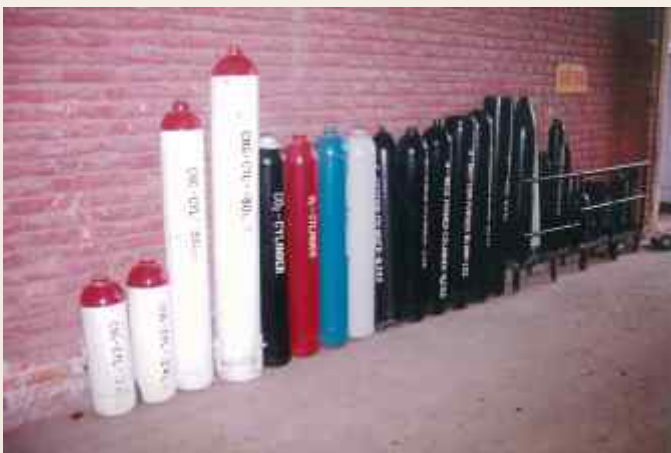
HP Gas Cylinders
